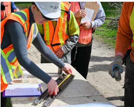
e. Logging core samples
