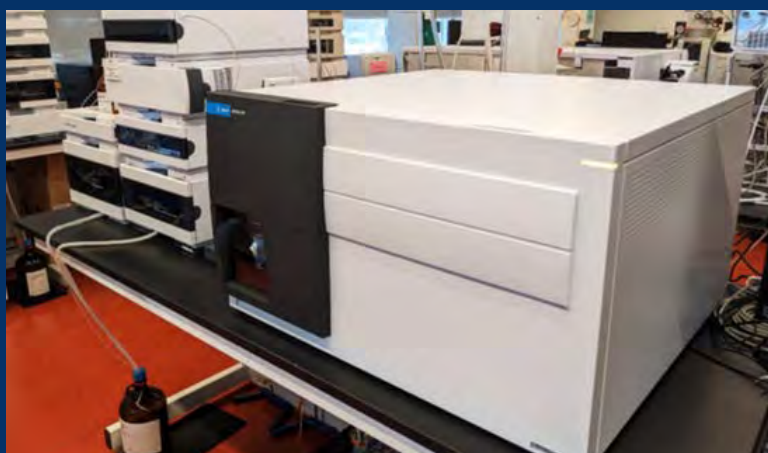
Picture 1. Agilent 6470 QQQ mass spectrometer connected to our ultra-high performance liquid chromatography (uHPLC) system.
