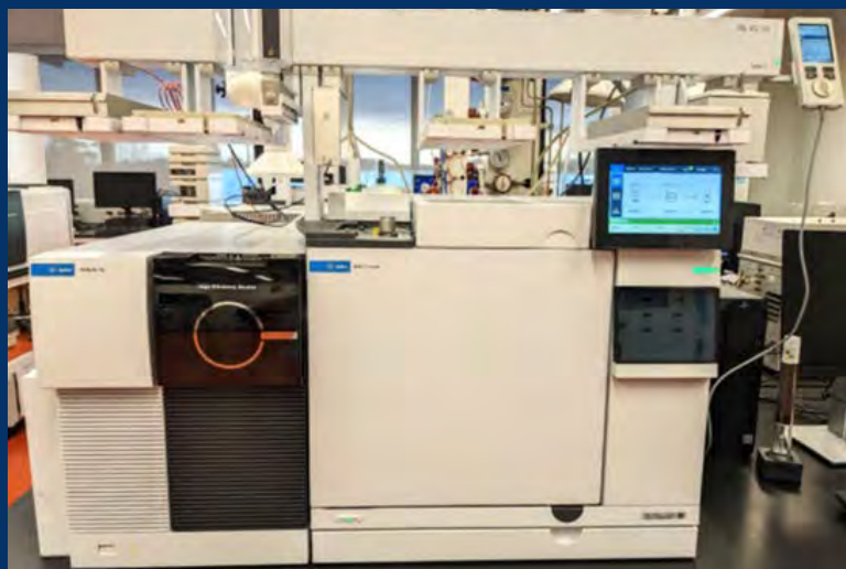
Picture 2. Agilent 7010B QQQ mass spectrometer connected to an 8890 GC system.
