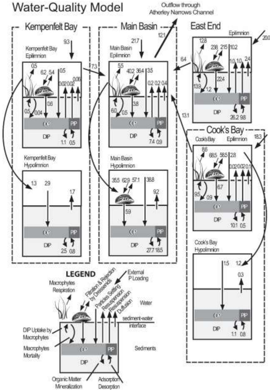
Figure 5. Simulated phosphorus fluxes (tonnes P year<sup>-1</sup>) in epilimnion, hypolimnion, and sediment layer at the seven spatial compartments of Lake Simcoe. The net TP contributions (sources or sinks) represent the mass of phosphorus associated with the various compartments (water column, sediments, macrophytes, dreissenids) averaged over the 1999-2007 period.
